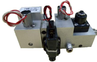
Integrated pneumatic valve system to control gas flow in an Anesthesia Ventilator
